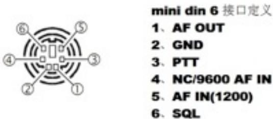
Pin 1. AF OUT, GW-1000 audio output to radio input
