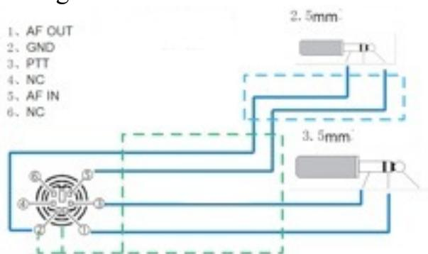
Mini din 6, pin 1 to the ring of 3.5mm jack (AF out)
